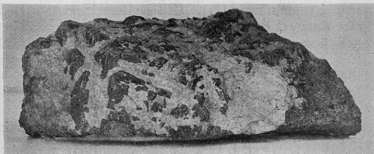
FIG. 2. CYRTOLITE (ALTERED ZIRCON) RICH IN HAFNIA, FROM NEAR BEDFORD, WESTCHESTER COUNTY, NEW YORK
